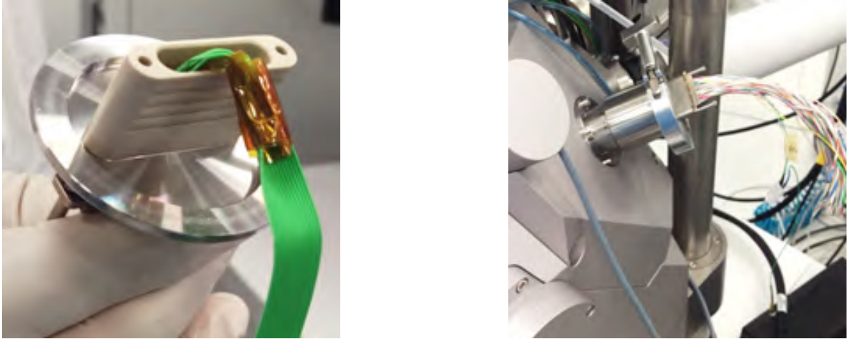
Figure 4.43: (Left) the cable connector from the detector. The components of the PCB and the solder are suitable for vacuum. (Right) the cable is connected via a wide reducer to the microscope.
